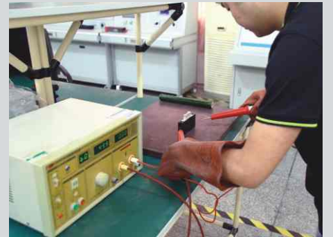
耐压试验 Withstand Voltage Test
