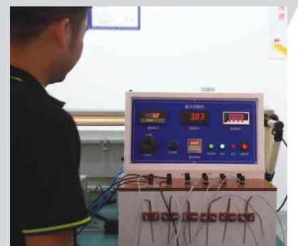
插件温升试验 Plug-in Temperature Rise Test
